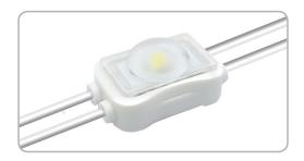
I2V LED modules with constant current. LED module diode life time depends on voltage fluctuations which appear in the circuit. Microprocessor which can be found in this new module, stabilizes current for each diode separately, so its lifetime becomes longer. Premium quality and even longer warranty period!
